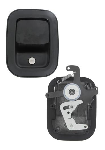
This flush mounted paddle handle with rigid locking paddle is a redesign of our popular 030-0850 Flush Mounted Paddle Handle. With a modernized look, it can be used in FMVSS 206 (ECE R11) applications, is power lockable and features a 4-point pivot plate and lock cam actuation.
